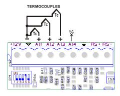
Reading of PT100/NI100 2wires or NTC-10K:
