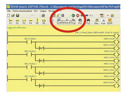
If the TD240 is connected correctly to the PC (see diagram of **section 4.1**), during the transfer the terminal will show this figure on the display:
