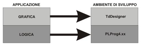
Any application managed by the TD240 terminal should therefore be realized using both the development environments, **implementing therefore two different files** strictly connected between them.
