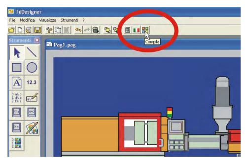
This operation is necessary to make the project available as soon as implemented to the development environment **PLProg 4.xx**. <u>The compilation has effect only if PLProg is open and the terminal</u> <u>TD240 has been selected as CPU.</u>
