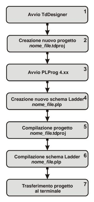
To create a new project and transfer it to the terminal, follow the procedure and described below:
