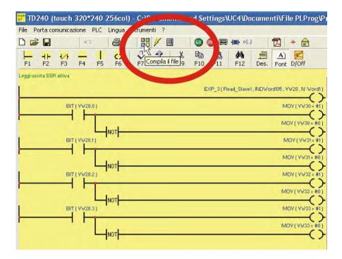
At this point, if saved by PLProg, file file\_name.plp will contain both the PLC part and the graphical part (is not necessary that the file .tdproj has the same name of the file .plp).
